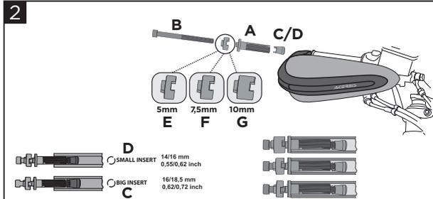
**insert the screw (B) inside the handguard, with the correct spacer (E/F/G) according to the type of bike (ensure that the throttle does not remain stuck on acceleration), then insert the expander (C) and the insert (C/D). Tighten all without locking and mount it on the bike. Verify the handguard's correct angle and tighten.**
