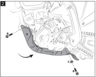
Position the fuel tank Acerbis (A) and screw first in front with two screws (B) without tightening them, then the other two screws (B) at the rear with the bushings (C) supplied. Finally close and tight all
